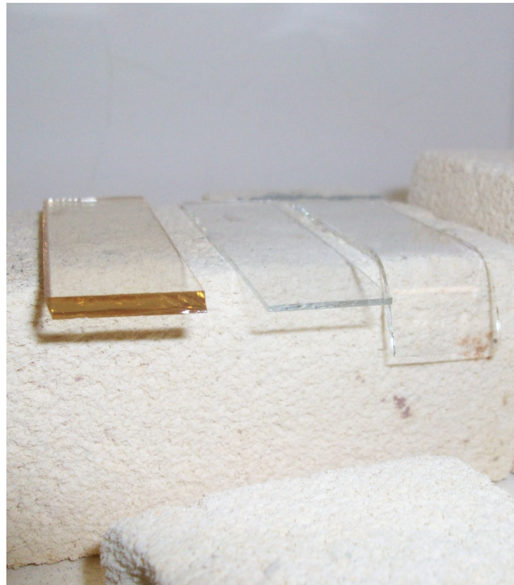
720 °C for 48 h One substrate unaffected, another bends slightly, another to a significant degree
