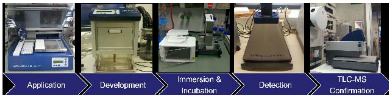
Workflow scheme of HPTLC-bioluminescence screening
