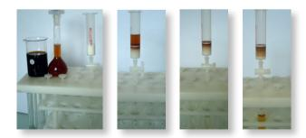
Tests with C18 reversed phase don't allow the recovery of total polyphenols content. Some polyphenols are eluted simultaneously with glycol. Only polymeric reversed phase is able to retain phenolic acids, flavan-3-ols or procyanidin polymers (condensed tannins).
