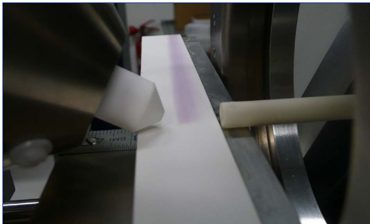
Visualisation for the HPTLC plate, treated with sugar solution + \beta -naphthol reagent
