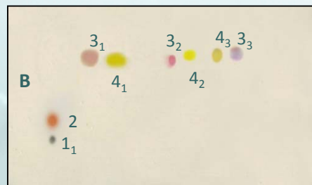
Separation of a pigments mixture of dyes for polymers by three-dimensional TLC
