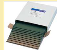
Plates selected are MERCK made of Silica Gel 60F 256 . Samples are applied with 2µl micro-capillaries
