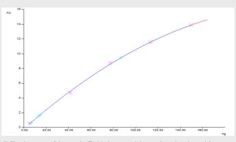
Calibration curve of the sample 'Fruitissimo' containing sucralose via polynomial regression (peak height) in the working range (1:30) of 5 ng to 150 ng. The calibration curve showed a coefficient of correlation of 0.9997.
