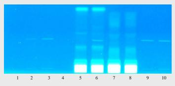
HPTLC plate image under UV 366/>400 nm illumination; track 1-3, 9, 10: sucralose standards (5 – 150 ng/band), track 4: blank track, track 5: fruit jelly extract ('Vitamin Wichtel', Natreen), track 6: standard addition of 9,6 mg/kg sucralose (80 ng/band) to the latter fruit jelly extract; track 7 and 8: fruit jelly extract ('Fruitissimo', Natreen).
