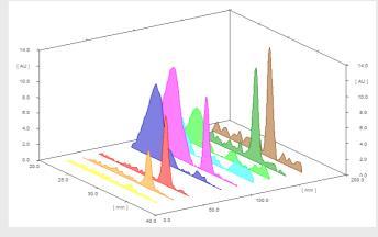
Analog curves obtained by fluorescence measurement at UV 366/>400 nm of sucralose standards and different fruit jelly samples; same track assignment as plate image (left).
