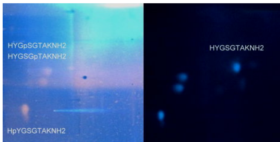
Two-dimensional HPTLC of a peptide mixture followed by Pro-Q® staining (left), and staining with fluorescamin (right)
